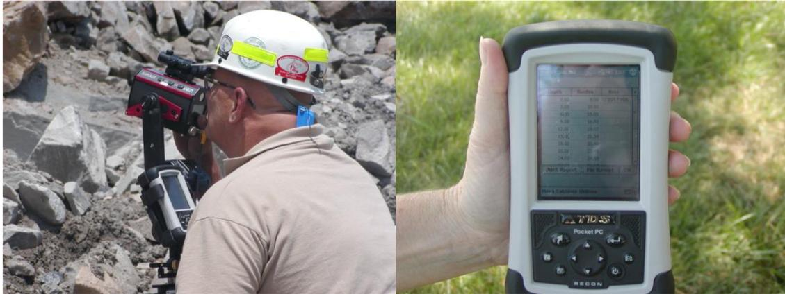
Figure 1 – 2-D Laser and Data Collector
