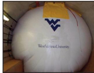
First RTC prototype for low inflation pressure
