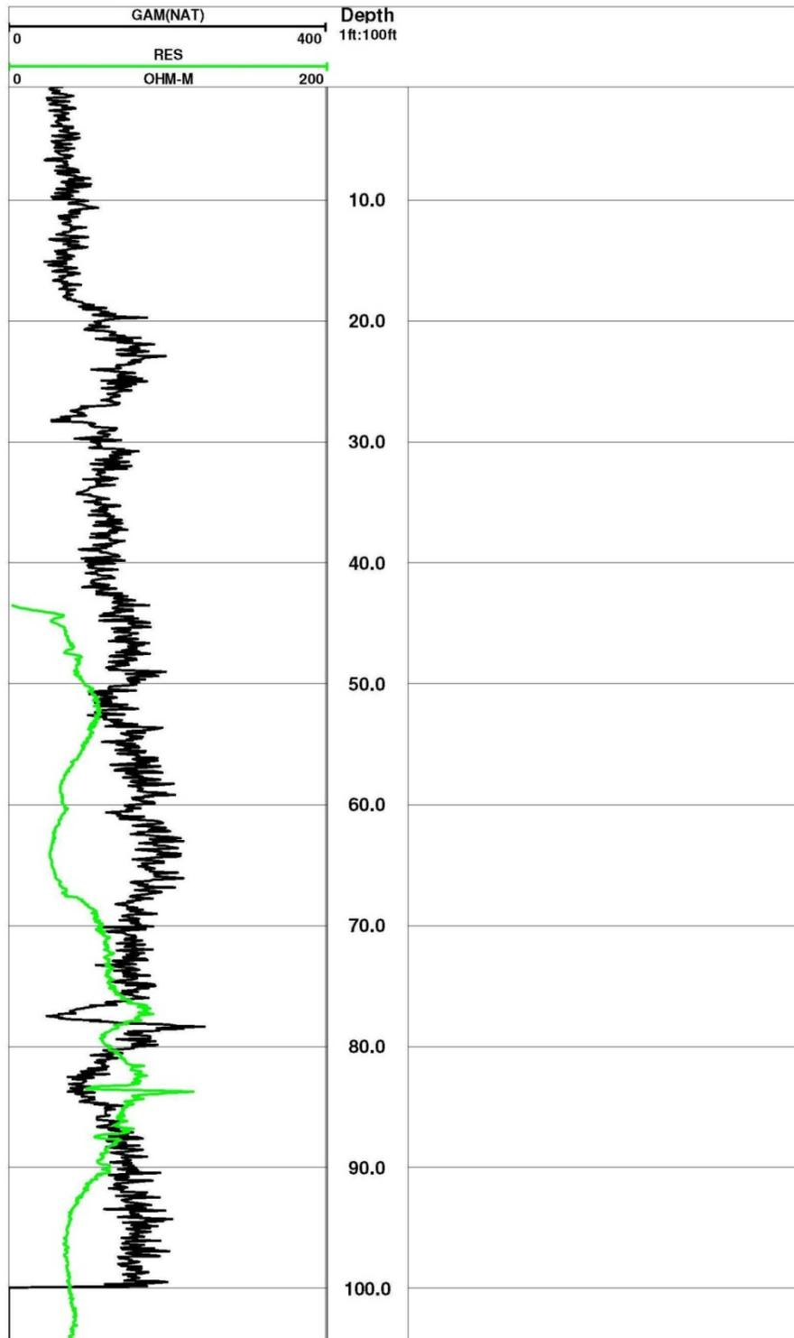
Figure 15: Kanawha County #0946 geophysical well log
