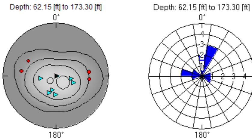
**Figure 17: Summary of fracture measurements for borehole Bar-0135. (A) Schmidt lower hemisphere polar plot of fracture dip, and (B) Rose diagram of fracture azimuth.**
