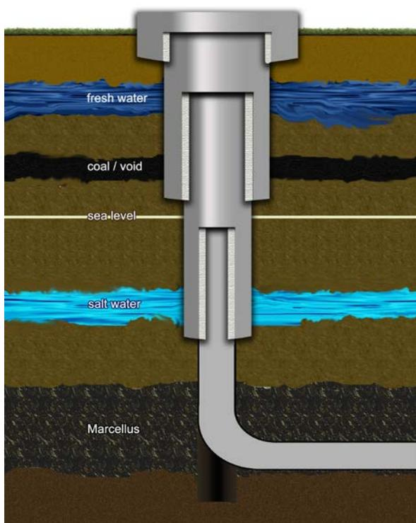
Figure 2-37 Generalized horizontal drilling
