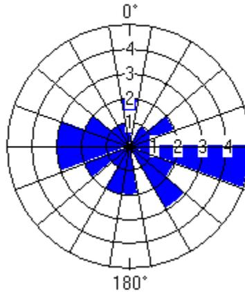
**Figure 13: Summary of fracture measurements for borehole Mng-0585. (A) Schmidt lower hemisphere polar plot of fracture dip, and (B) Rose diagram of fracture azimuth.**
