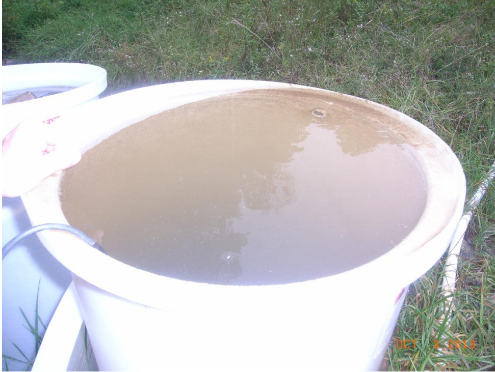
Figure 4: Solids accumulation in the control treatment unit
