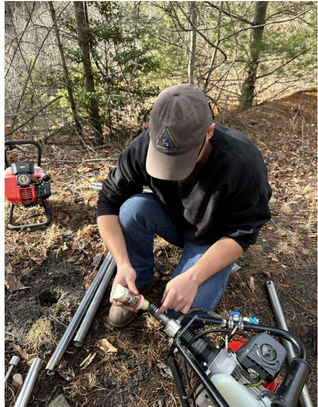
A WVGES geologist prepares the backpack core drilling unit to collect samples in the field.
