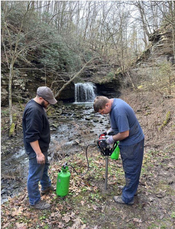
Two WVGES geologists collect core samples using the backpack core drilling unit.
