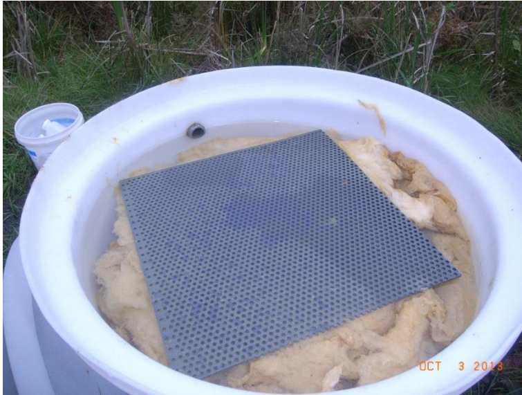
Figure 3: Fiberglass insulation media (grate to hold insulation in place)
