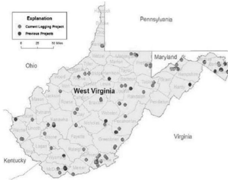
Figure 3. Location of USGS-WVDEP borehole geophysics well logs 2014-2018. Water Use Section - Mine Pool Study
