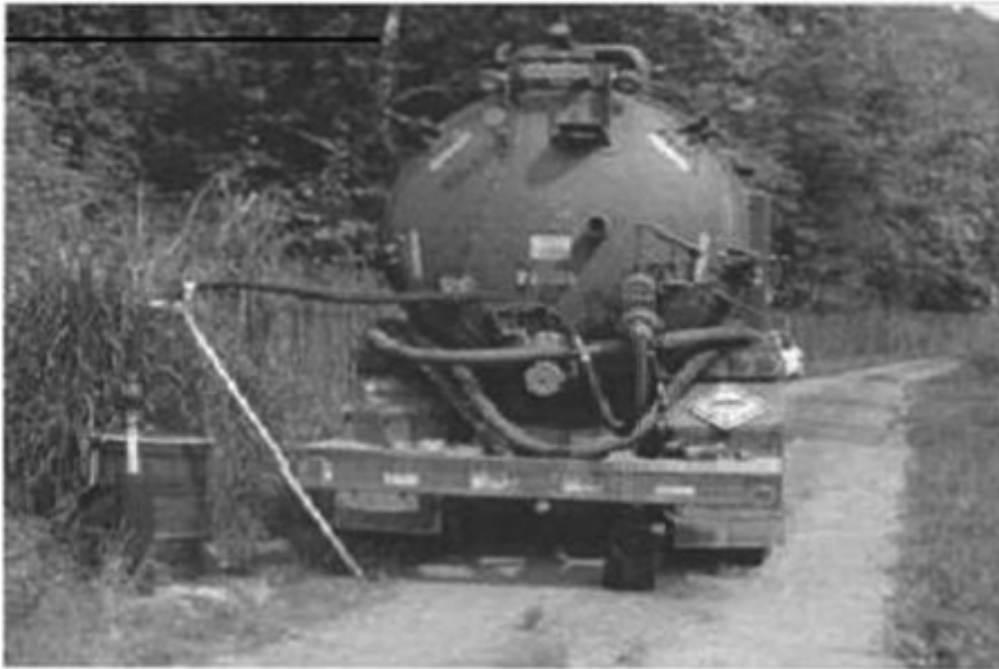
Above, a Geoprobe unit injects oxygen release compounds at a bio-remediation site. Below, a high vacuum pump truck extracts hydrocarbons.
