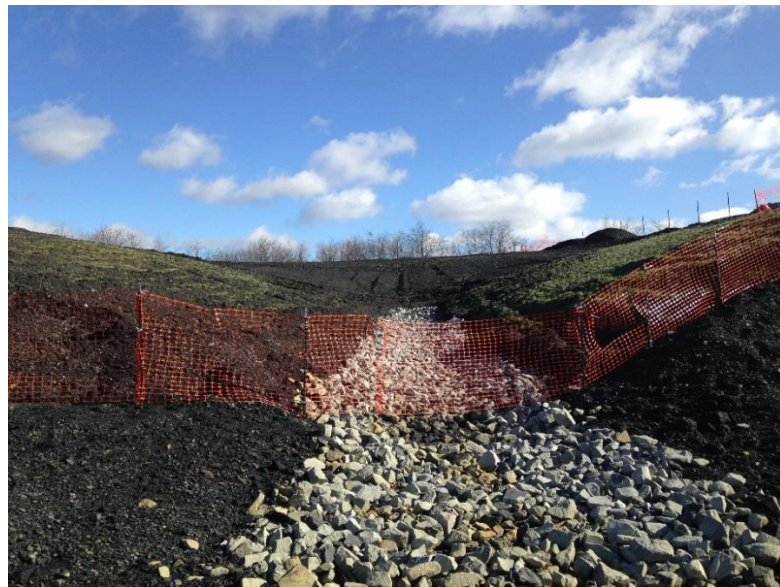
Figure 6 Test plots with early vegetative growth; 60:40 mix left side, 80:20 right side, and no residuals applied in the middle.
