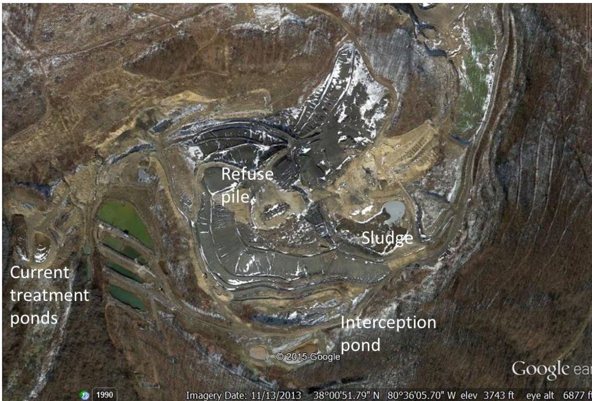
Figure 1. Coarse coal refuse pile
